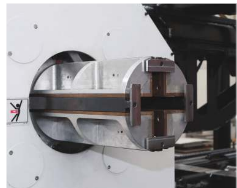
■ Thanks to its high-strength clamps, it ensures that the material hold prepared for cutting accurately and precisely. (S)
