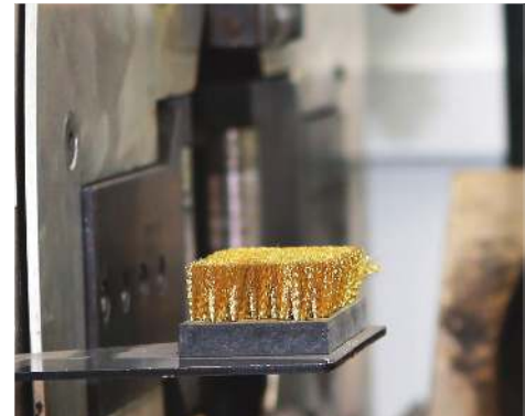
■ This is used for automatic cleaning of the nozzle that was contaminated during the cutting processes of materials. (S)
