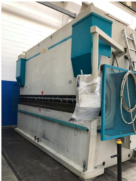
**PRESSA PIEGATRICE IDRAULICA SINCRONIZZATA "BL" USATA**, LUNGHEZZA DI PIEGA 4100mm, POTENZA 200TON, 4 ASSI, CNC ESA KVARA DUEMILA4, VERRANNO MONTATE FOTOCELLULE DSP, POTENZA 19,8KW, ANNO 2006, S.N. 01006/049, CE
