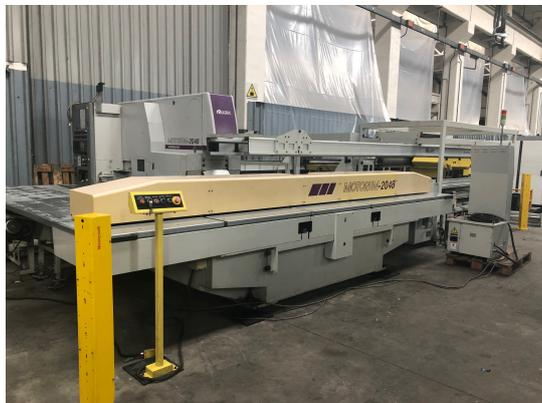
PUNZONATRICE ELETTRICA A TORRETTA "MURATEC-WIEDEMANN" USATA MOD. M2048 , COMPLETA DI CARICO/SCARICO AUTOMATICO MOD. F1250, ENTRAMBI ANNO 2000, TORRETTA A 30 STAZIONI COMPRESI N.1 MULTITOOL E N.2 INDEX, SPESSORE MAX PUNZONABILE 6mm, CAMPO DI LAVORO 1250x2500mm, POTENZA 20TON, 19.000H DI ACCENSIONE, CNC FANUC, CE, INGOMBRO TOTALE CIRCA 15000mm
