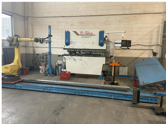
**CELLA ROBOTIZZATA FARINA/STARMATIK** COMPOSTA DA: PRESSA PIEGATRICE SINCRONIZZATA "FARINA" MOD. PSN 40/20 ANNO 2000 + ROBOT "FANUC" MOD. M710IC/50 +
