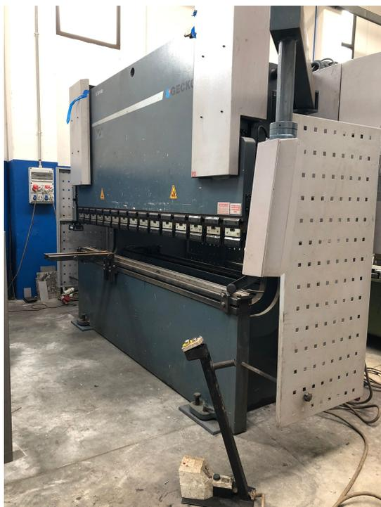
**PRESSA PIEGATRICE IDRAULICA SINCRONIZZATA "GECKO" USATA**, MOD. E30160, LUNGHEZZA DI PIEGA 3050mm, POTENZA 160TON, 4 ASSI, FOTOCELLE DI SICUREZZA DSP NUOVA ELETTRONICA, CNC CYBELEC, CANCELLO POSTERIORE DI SICUREZZA, CORSA 200mm, ANNO 2007, 15 KW, S.N. 7531072154E, PESO 9820KG, DIMENSIONI 4200X2100XH2700mm, CE
