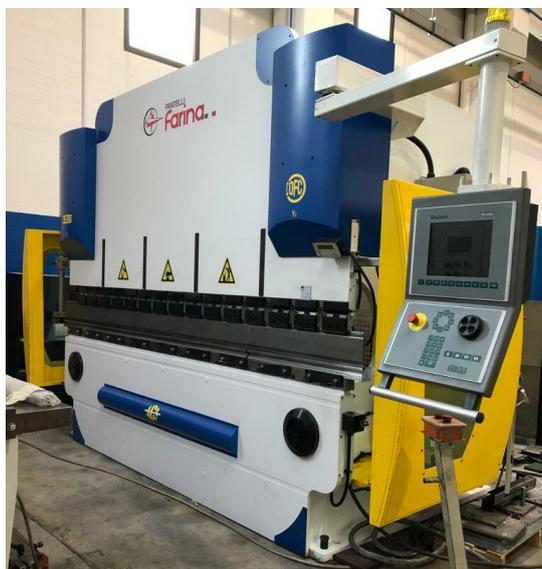
PRESSA PIEGATRICE SINCRONIZZATA "FARINA" USATA, MOD. PSN 110/30, LUNGHEZZA DI PIEGA 3100mm, POTENZA 110TON, 6 ASSI (Y1,Y2, X, R, Z1, Z2) BOMBATURA IDRAULICA, PACCHETTO PLATINUM (BOMBATURA ATTIVA, TMS E DFC), CONTROLLO NUMERICO DELEM DA 65 W, BLOCCAGGIO PNEUMATICO SUPERIORE, INCAVO 500MM, N.4 PUNTALI (2 AUTOMATICI E 2 MANUALI), FOTOCELLULE LAZER SAFE, ANNO DI PRODUZIONE 2006, MATR. 4280306/P, CERTIFICATA CE, 15 KW, 9440 KG
