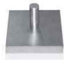
■ 12 mm hole cuts with True Hole Technology
