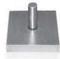
■ 12 mm hole cutting without True Hole Technology
