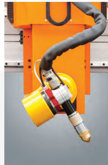
■ Can move totally +50 and 60° degrees at B axis.
